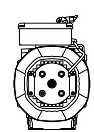
tolerances: ½: ±½6" .xx : ±0.010 **Gearmotor Specifications** Gearmotor Current Rating 14.6A Gearmotor Voltage 230VAC 60hz 3ph drawing is the Gearmotor Brake Voltage 230VAC 60hz 1ph Motor Output Torque | 4280 lb-in 73RPM @ 60Hz, max 146RPM @120Hz Motor Output RPM Encoder PPR 1024
