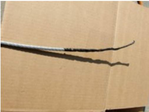
Step 3. Now the cable can be guided through the cable slot in the dog. One final suggestion is to run something (fish-tape, tie-wrap, coat hanger, etc...) through the slot from the other direction, tape it to the tapered cable and pull it back through.
