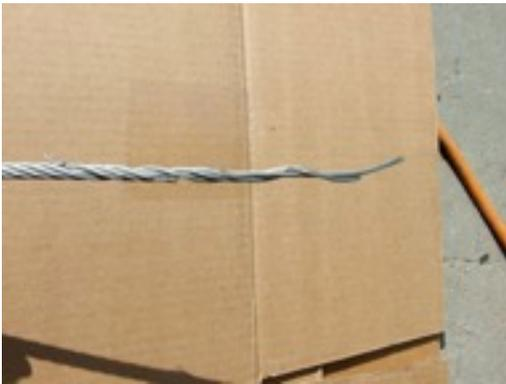
Step 2. Wrap electrical tape around the tapered end, starting at the end and working down past the last cut. Be careful to fold the cut ends back into the cable when taping. When finished, the cable should look like this:
