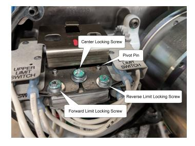
When both screws on one plate are loosened, you can pivot the limit on an indexing pin, moving the initial limit closer or farther away from the ultimate limit.
