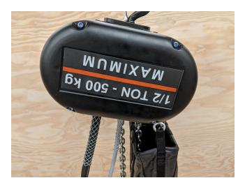
These screws need to be loosened to take the limit enclosure hood off and access the inside of the **Smart Chain Hoist.** To open the **Smart Chain Hoist**, you will need a 3/16" Allen key. Be aware, each hood has a gasket which must be reseated properly.
