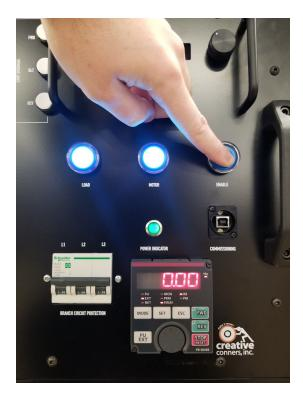
While holding the Brake Test Button, press the Load Brake button. This will manually release the Load Brake. The Motor Brake should still be engaged and will hold the load. If the suspended scenery slips down, release the Load Brake button immediately. Since the Motor Brake did not hold the load as expected, that brake has failed. DO NOT OPERATE THE MACHINE UNTIL THE MOTOR BRAKE IS REPAIRED OR REPLACED. FAILURE TO REMOVE THE MACHINE FROM SERVICE COULD RESULT IN DAMAGE, INJURY, OR DEATH.
