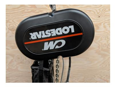
Like the limit enclosure, you will need to loosen the two screws with a 3/16" Allen Key. Once taken off, you will see the motor and signal wiring, as well as the motor and speed encoder.
