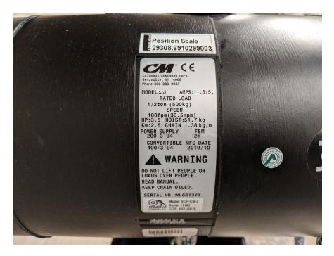
This number will need to be set in the Position Scale field in Spikemark. If you are having trouble with the scaling on your **Smart Chain Hoist**, you can calculate and adjust either by using our Position Scale Wizard or by calculating the math yourself.
