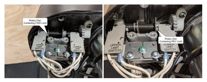
Once set, place the capture plate back into position, indexing with the rotary discs, and tighten the 5/32" screws. Once you test that the limits are engaging where you want them, you can replace your limit hood onto the hoist enclosure.
