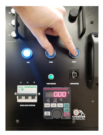
• Release the Motor Brake button
