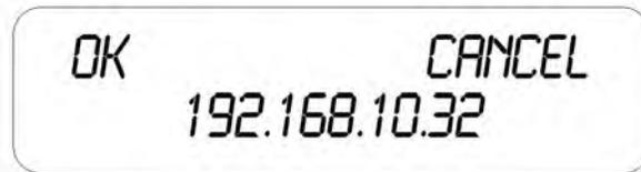
3. By turning the knob, move the cursor over the segment you wish to change. In this example, move the cursor until it is flashing over the number "32".
