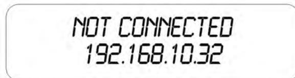
“Not Connected” indicates that the Stagehand FX is not communicating with a computer running **SpikeMark**.
