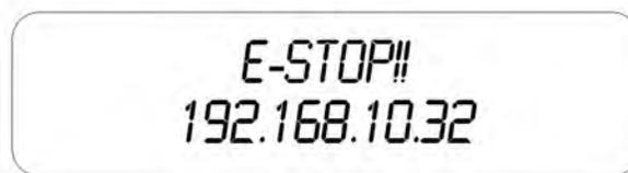
The “E-Stop!!” message is displayed because you have not yet hooked up the Stagehand with Showstopper. If the Stagehand does not detect a signal from Showstopper, it will assume an Emergency Stop condition.
