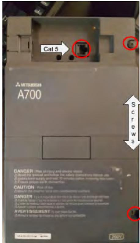
9. Plug the cat5 cable back into the VFD.
